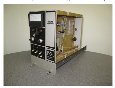
CAM stations, the analyses of the multi-gas bubbler solutions and weighing the increased number of high volume air sampler filters. The CAM station instruments and the multigas bubblers all used wet chemistry techniques to absorb pollutants into chemical solutions. The solutions were analyzed for pollutant concentrations using colorimetric analyses.
