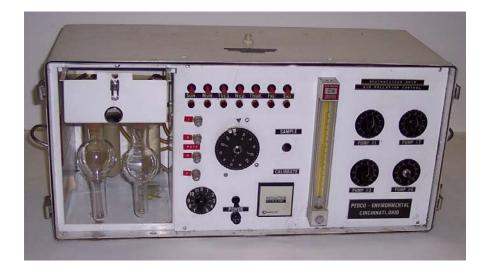
Then there was the addition of six CAM stations. These Continuous Air Monitoring Stations (CAM) were specially modified mobile homes that housed instruments to monitor seven air pollutants on a continuous basis. The CAM stations also contained meteorological instruments that collected data continuously. Each station required an operator to maintain the instruments and to collect the huge volume of data generated. Each CAM station cost approximately \$100,000. The CAM station located behind Drake
