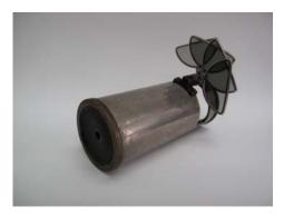
The umbrascope consisted of four grey lenses which could swing in and out of view, allowing the inspector to look at the smoke through varying shades of grey. When emissions could be seen through all four lenses of the umbrascope, then the smoke was dark enough to be in violation of the ordinance. If violations persisted, the proprietor could be fined \$25 to \$100.
